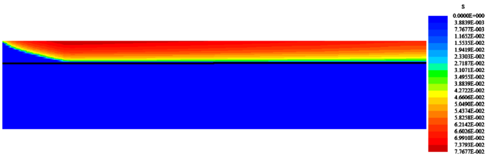
Fig. 7.8. Liquid water-saturation when C_{in} = 14 \text{ mol/m}^3, u_{in} = 2 \text{ m/s}, I = 1.5 \text{ A cm}^{-2} . The evaporation front separating the two-phase zone from the single-phase region is approximately represented by s = 0.03 .
